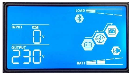
Night Time – Battery powering the loads
